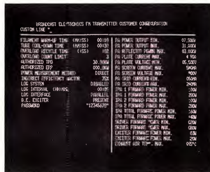
Broadcast Electronics' MVDS system screen display. Shown here is page three, the "Customer Configuration" screen, with which the user determines allowable maxima and minima for all monitored functions.
